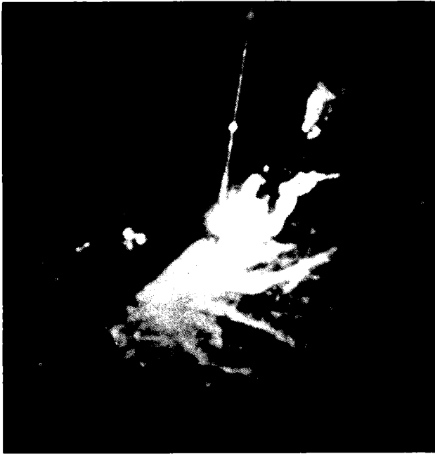
FIG. 6-11.—Photograph of the PPI on a 1.25-cm system, showing the striated appearance of the sea echo. Range markers are 1 mile apart. The bright line is the north heading.
