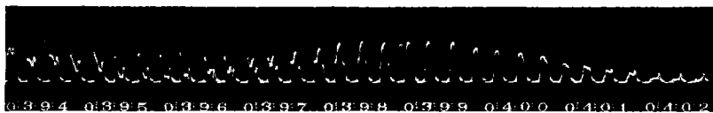
FIG. 6-34.—Section of the pulse-to-pulse record of the echo from a battleship on 9.2 cm. Pulse-recurrence frequency 333 pps, pulse length 1 \mu sec.
