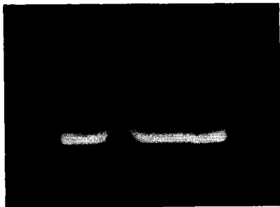
FIG. 7.2.—Photograph of precipitation on an A-scope with a 10-mile sweep. Most of the detail is lost, but the characteristic "fuzzy" appearance is still partly visible.
