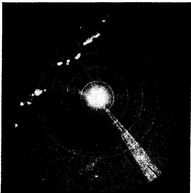
FIG. 7-9.—A line of thunderstorms in a cold front as shown on the PPI of a 3.2-cm radar system at the Radiation Laboratory on July 22, 1943. Beamwidth is 1.5^\circ , pulse length 1 \mu\text{sec} ; and the range marks are 20 miles apart.
